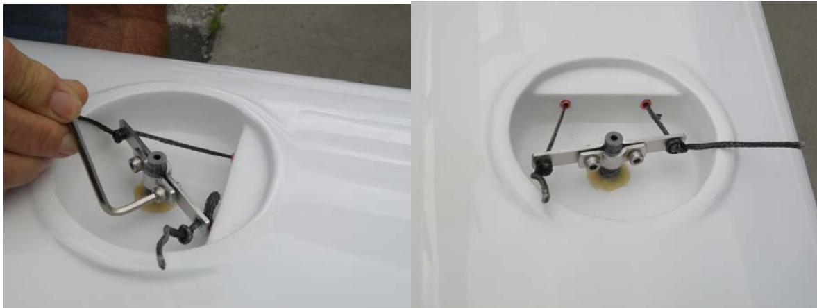
Photo 9. V-Series – once spreader bar is over the top of the rudder post, use allen wrench to tighten the spreader bar bolts so that top of rudder post and pin ends are pinched and held fast
