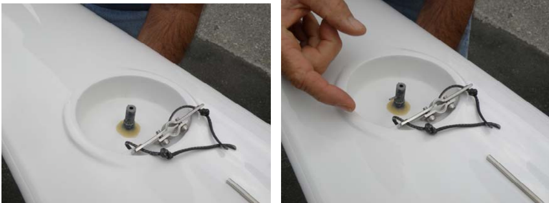
Photo 5. V-Series – run rudder post up through rudder housing in hull of boat
