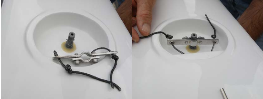
Photo 7. V-Series – center rudder pin in rudder post
