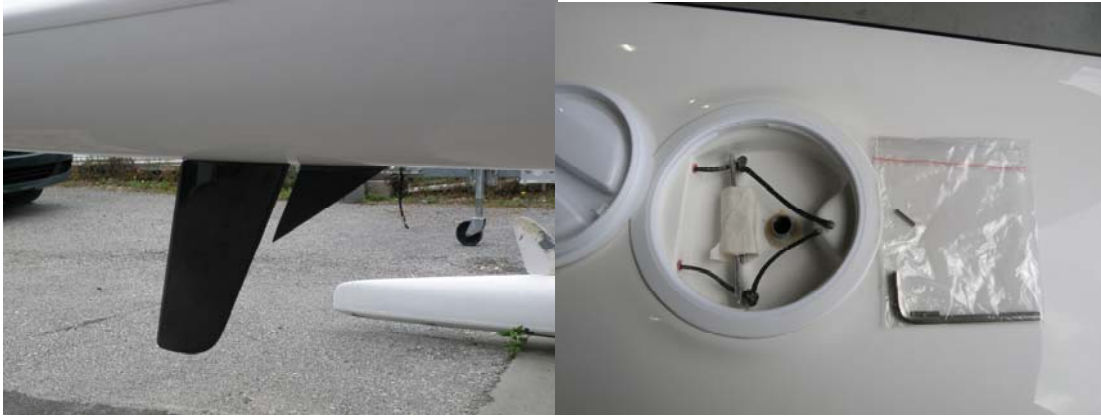
Photo 3. V-Series – installed Universal rudder and weed guard
