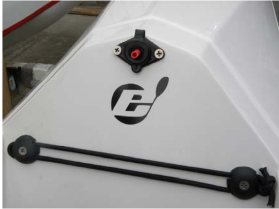
Photo 13. V-Series – footwell bungee and drain plug/breather tube in closed position
